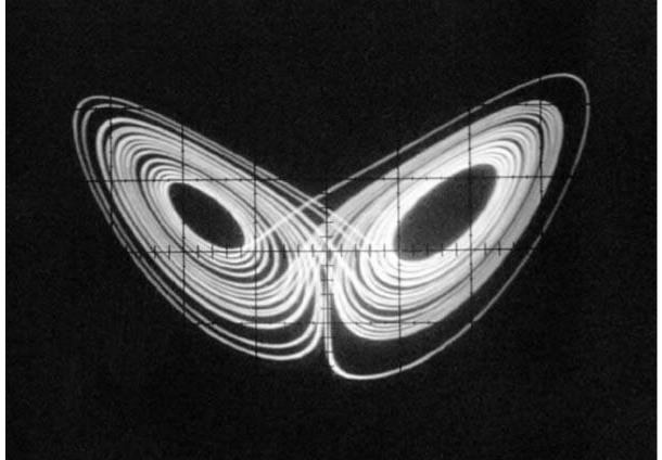
...the characteristic "owl's face" of the Lorenz attractor. The curve plays out in time, sometimes appearing to hesitate as it scales the boundary and decides which basin to drop back into. The value of C, the three integrator capacitors, sets the time scale: at 0.47uF it does a leisurely wander; at 0.1uF it winds around like someone on a mission; and at 0.002uF it is fiercely busy solving its equations and delighting its audience.
