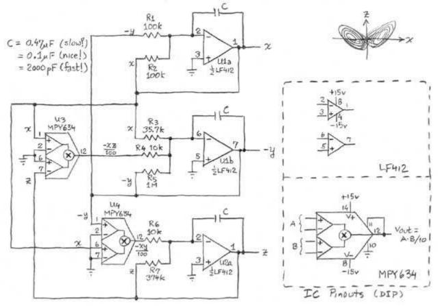
It's not hard to understand: the op-amps are wired as integrators, with the various terms that make up each derivative summed at the inputs. The resistor values are scaled to 1 megohm, thus for example R3 weights the variable x with a factor of 28 (1M/35.7k); this is combined with -y and -xz, each with unit weight. (note: the equations on the diagram are normalized to 0.1V, hence the multiplier scale factor of 100.)
